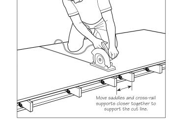
• Use for any task where a sacrificial work stand-off is needed: cutting, drilling, clamping, finishing, etc.
